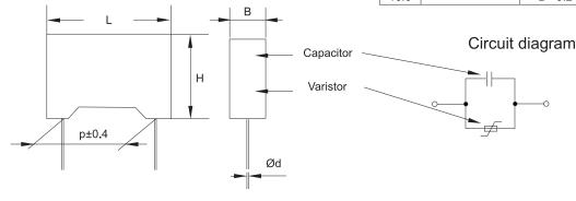
The F5A Series was designed for different suppression conditions and peak voltage limitation. Different operating and clamping voltages allow an optimal adaption to the different application requirements. Best results for suppression purposes are achieved by using low inductive MKT capacitors in parallel construction with ceramic varistor in one single case. The leaded EMI-RFI suppression element F5A is mainly prepared for Automotive applications without PC-board (e.g. motor
